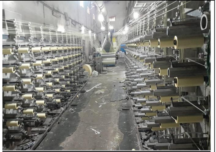
**Weaving or Circular loom process:** In this process, the tapes are pulled from bobbins with the help of weaving machines. The circular loom runs on a very high speed. The requirement of bobbins differs according to different shuttles and use of these shuttles depends on the type of fabric desired. These fabrics are in circular form and is then rolled on a big roller and such rolled fabric can either be directly put on to the cutting machine or be laminated as per requirement of customer.
