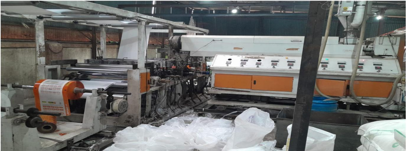
**Cutting process:** The fabric is cut according to the dimensions required by the customer. Cutting of fabric can be done at the time of rolling it on the roller or after lamination process. In this process the fabric in the rolled form is passed through cutting machine and measurements for cutting the roll or the sheets are inserted in the machine and the output is fabric sheets which can be used either in the printing process or directly in stitching process.
